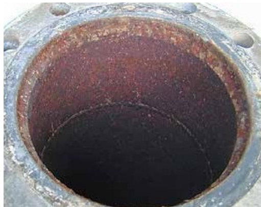
The pipe is almost clogged with scale.
