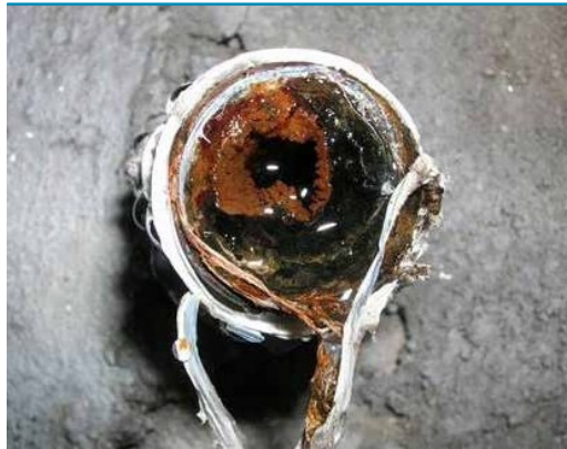
The pipe is almost clogged with scale.
